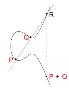
Figure 2 Elliptic Curve Point addition[18]
