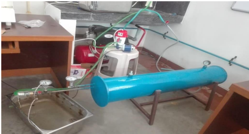
Figure 2 Shell and tube Type heat exchanger
