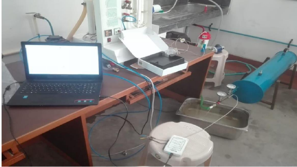
Figure 3 Shell and tube type Heat exchanger with DAQ set up
