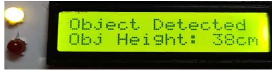
Figure 1.10: Object height measurement
