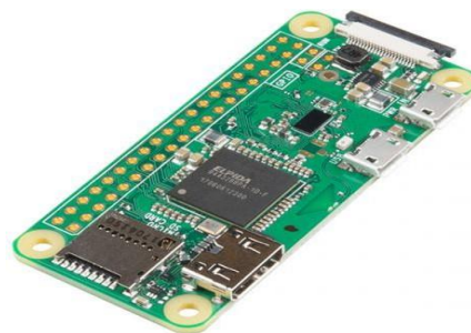
Fig. 3 Raspberry zero w RASPBERRY PI CAMERA
