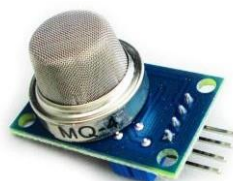
Fig. 6 MQ-4 Gas Sensor DHT11 HUMIDITY SENSOR
