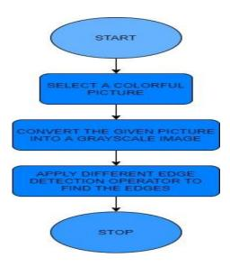
The proposed approach of the flow chart is given as at the intial stage a colorful picture is picked and embedded into the software like MatLab In which processing of pictures takes place. The picture is changed over into grayscale in the following step. A gray scale picture is mostly a mix of both black and white color.
