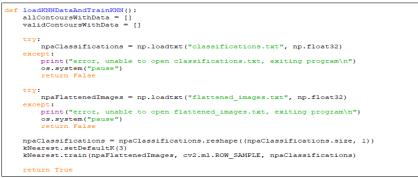
Figure 4.3.1. Pseudo code for loading KNN algorithm
