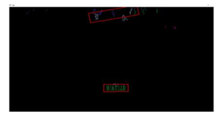
Figure 5.7. Image highlighting the region having a possibility of a number plate
