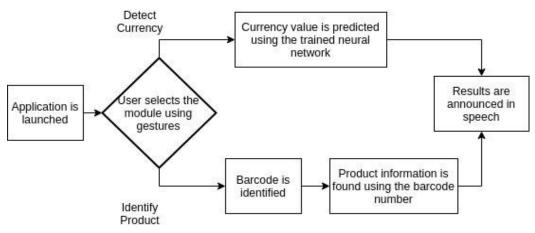
Figure 1. System Workflow
