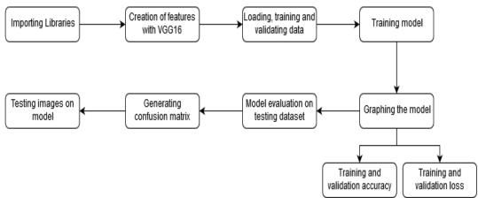
Figure 1. Design of proposed neural network
