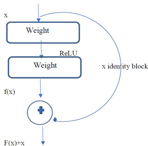
**Fig 2. Single Residual RD block: A block diagram**
