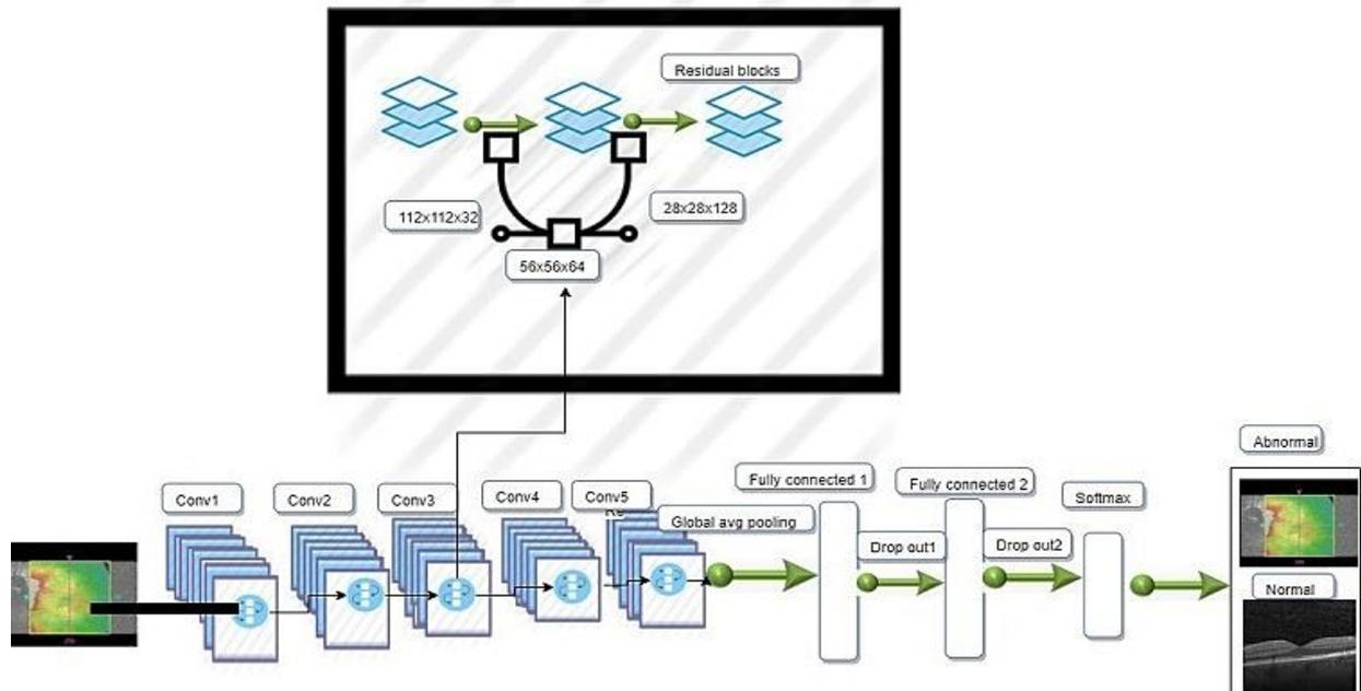
**Fig 1. Residual RDnet architecture**
