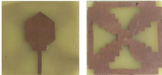
**Fig. 9** Top and Bottom view of fabricated prototype antenna
