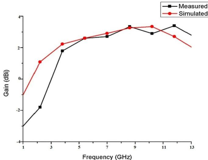
**Fig. 12** Gain (dBi) w.r.t frequency plot for designed patch antenna
