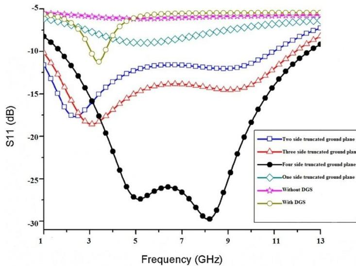
**Fig. 8** Return loss for parametric variation of ground
