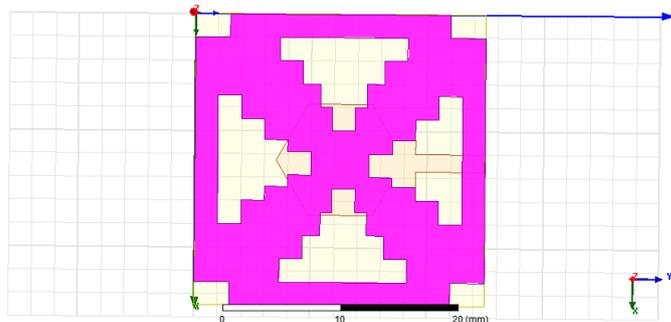
**Fig. 2** Modified hexagon-shaped patch antenna ground plane
