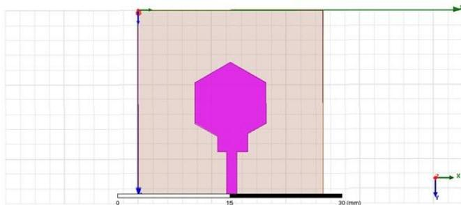
**Fig. 1** Modified hexagon-shaped patch antenna radiator
