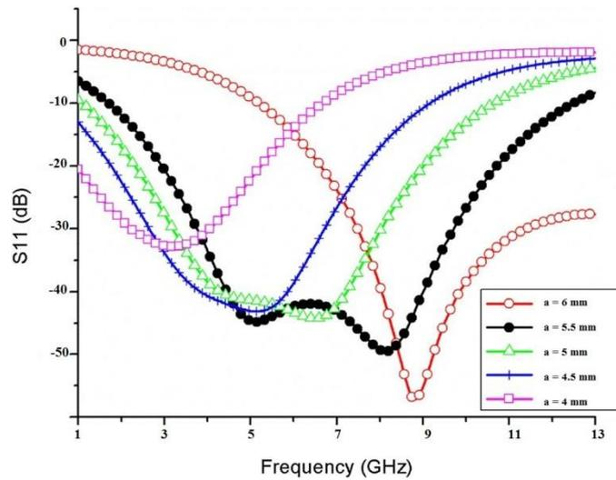
Fig. 5 Return loss for parametric variation of hexagon side length
