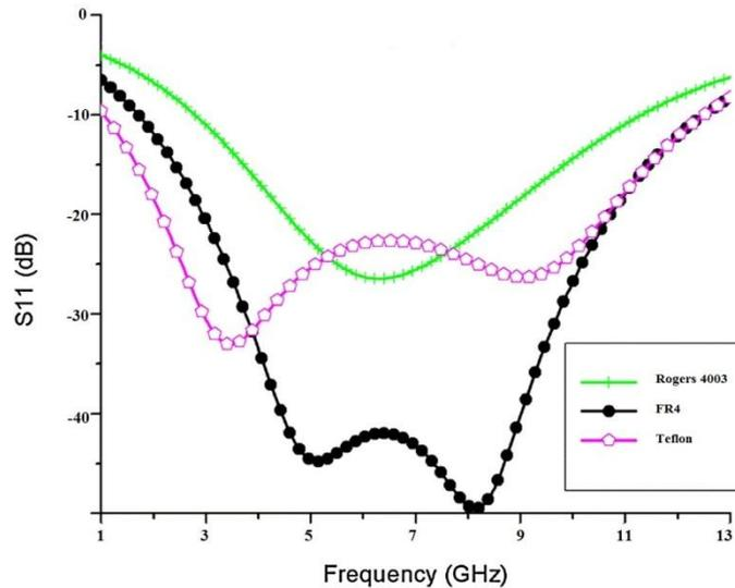
**Fig. 7** Return loss for different material
