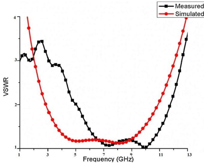
**Fig. 11** VSWR w.r.t frequency plot for designed patch antenna
