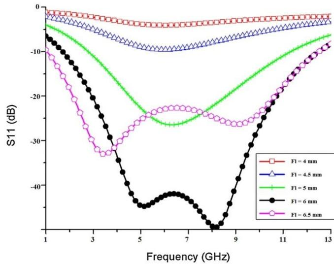
Fig. 4 Return loss for parametric variation of feed length
