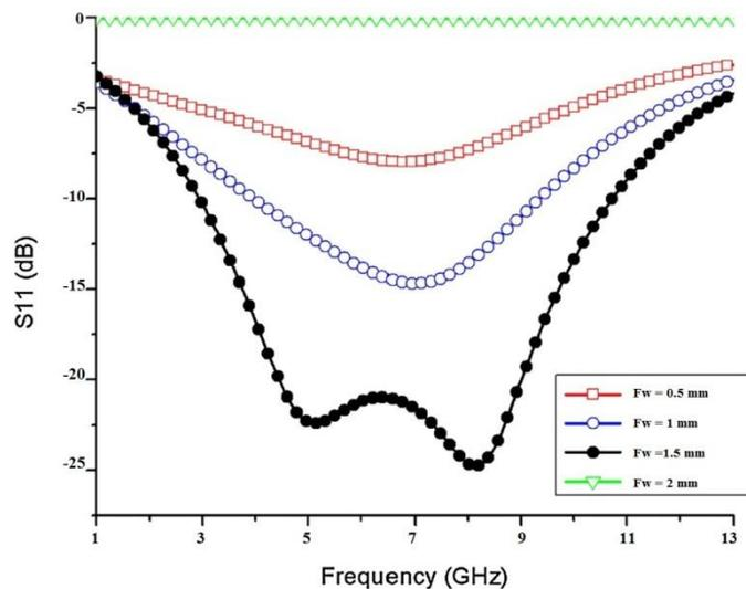
**Fig. 3** Return loss for parametric variation of feed width
