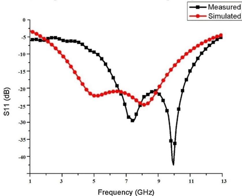
**Fig. 10** Return loss w.r.t frequency for designed patch antenna
