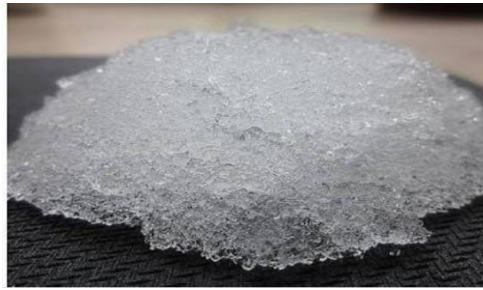
Fig. 2 SAP after addition of water
