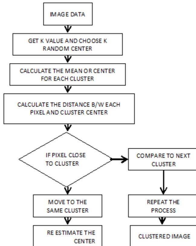
Fig. 2. K –means clustering algorithm
