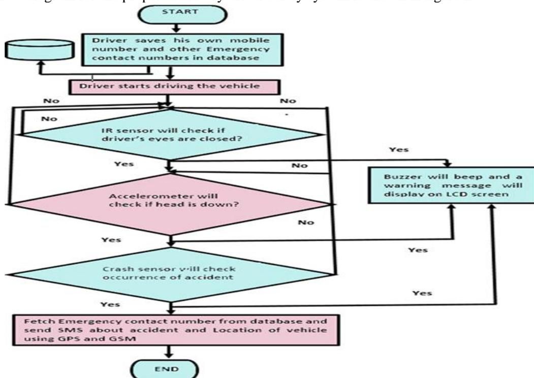
Figure 2: Flow diagram of the Proposed Drowsy Driver Safety System
