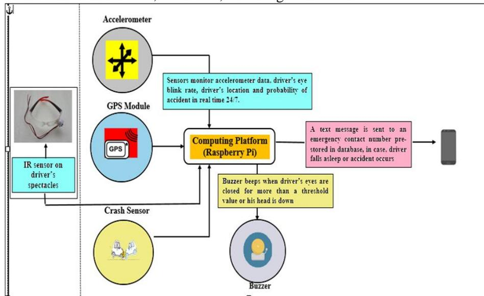
Figure 1: Architecture Diagram of the Proposed Drowsy Driver Safety System
