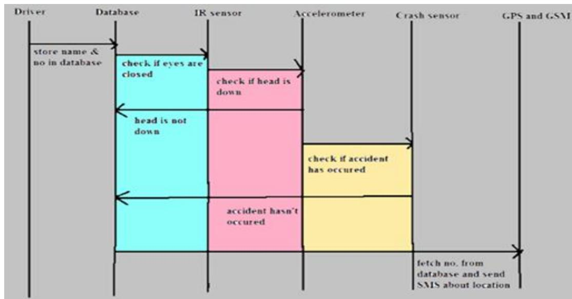
Figure 3: State Transition Diagram for Proposed Drowsy Driver Safety System
