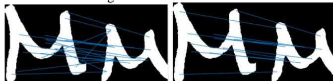
Fig. 6: (A) SIFT key points and matching, blue lines showing key points correspondence (B) Pruned SIFT key points and matching, blue lines showing key points correspondence
