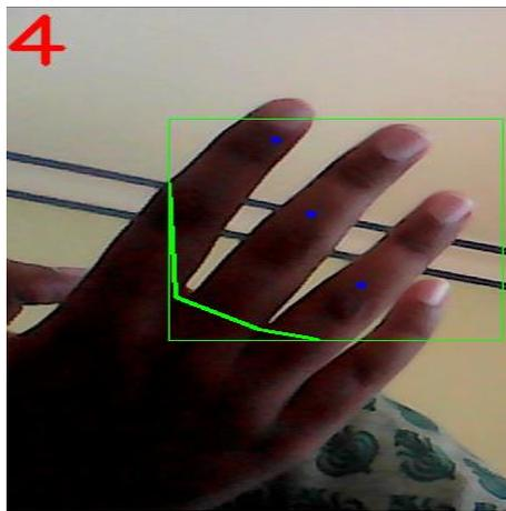
Fig.10 Identify four fingers in the region of rectangular box
