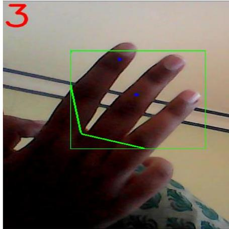
Fig.9 Identify three fingers in the region of rectangular box
